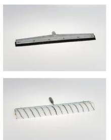
With a few exceptions (e.g. MC-DUR 1365 HBF), primers are applied by pouring and then spreading with the rubber squeegee, followed by levelling and equalising with a lambskin roller to avoid puddle formation. The consumption level is usually around 300 g/m<sup>2</sup>.
